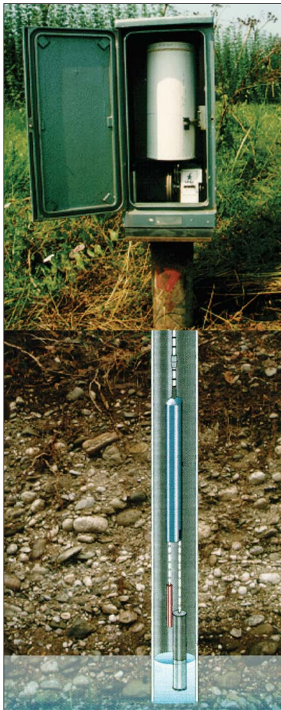
Shema merilnega mesta v Levcu v Spodnji Savinjski dolini. Observation well at Levce in the Lower Savinja valley.
