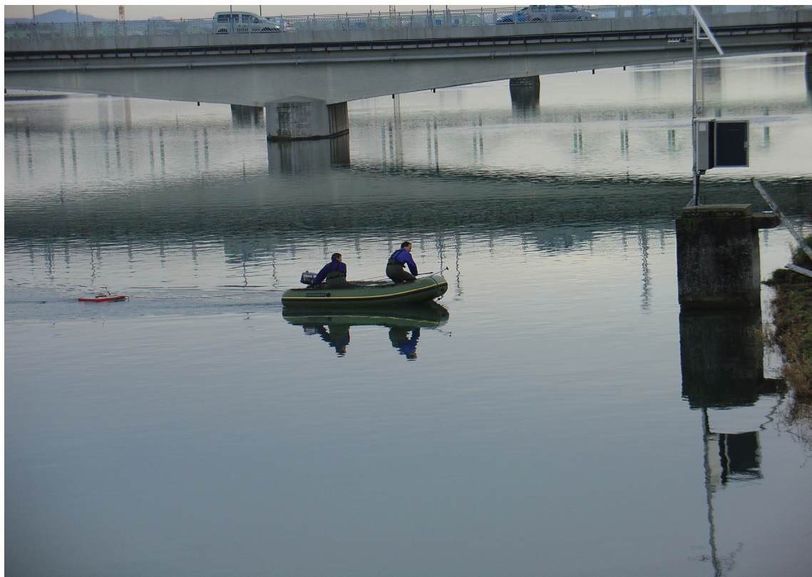
Izvajanje meritev pretoka na v. p. Ptuj – Drava. Na desni strani opazimo merilno mesto s podstavkom za sonde, omarico s komunikacijsko opremo ter drogom za anteno in solarni panel (foto: Roman Trček). Performance of discharge measurements at the Ptuj g. s. - the Drava River. A gauging site with a plate for probes, cabinet for communication equipment and a bar for the antennae and solar panel is on the right (photo: Roman Trček).
