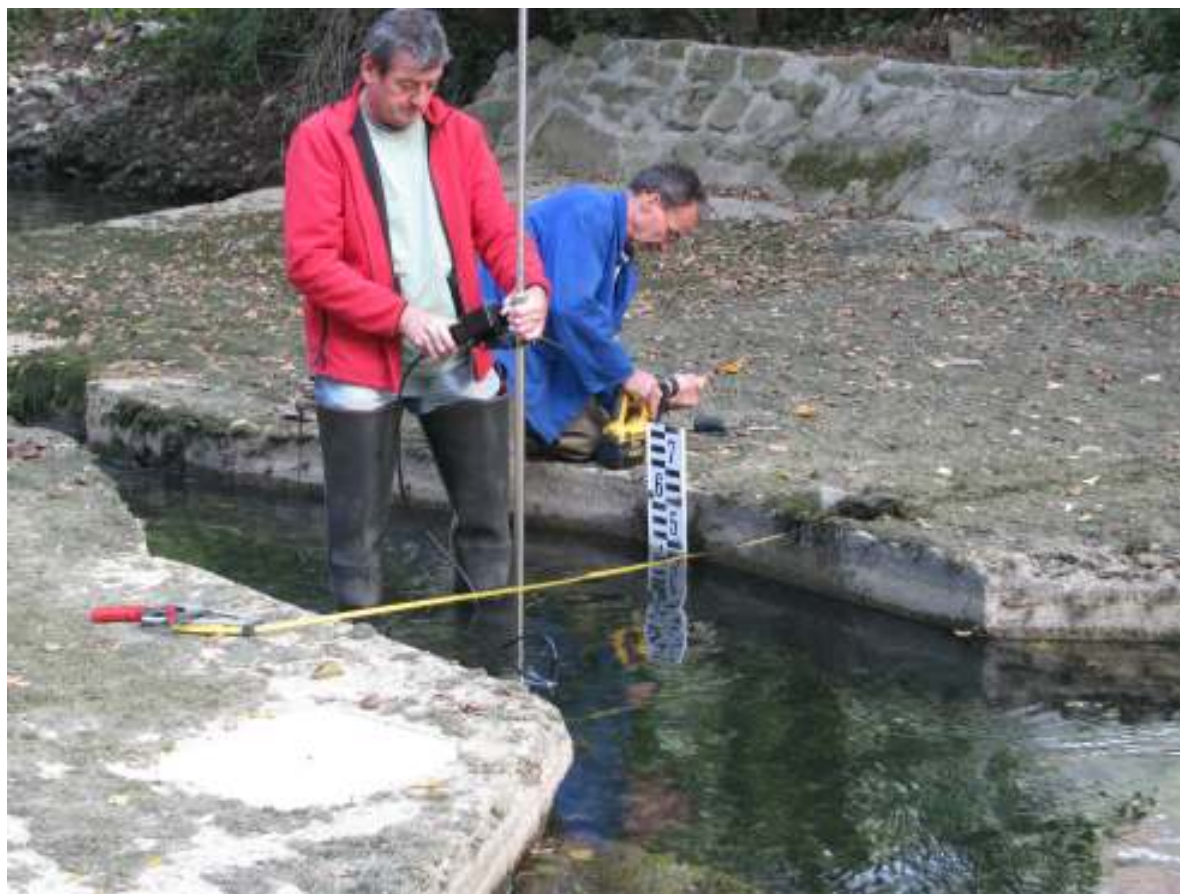
Slika 5. Izvajanje meritve pretoka ob nizkem vodnem stanju septembra 2009 (foto: Arhiv ARSO) Figure 5. Measuring of discharge on gauging station Kubeč during low water in September 2009 (photo: Archives of ARSO)
