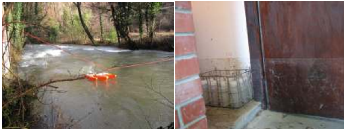
Slika 4. Izvajanje meritve pretoka visoke vode marca 2009 (levo) in sled visoke vode kot najvišje zabeležene gladine v obdobju opazovanj, 18. septembra 2010 (desno) (foto: Arhiv ARSO) Figure 4. Measuring of discharge during high water in March 2009 (left) and trace of the highest registered water the period, September 2010 (right) (photo: Archives of ARSO)
