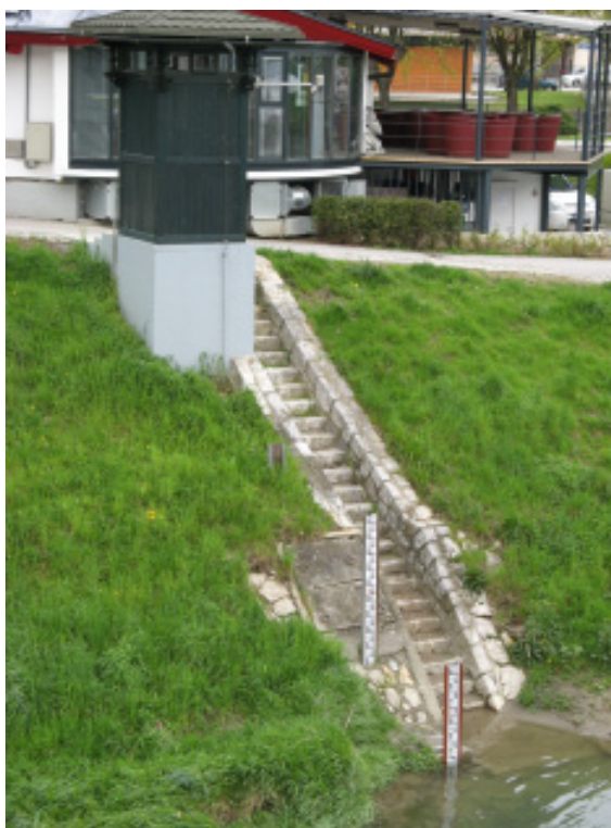
Slika 3. Vodomerne postaja Laško na Savinji (foto: Arhiv ARSO) Figure 3. Gauging station Laško on the Savinja River (photo: Archives of ARSO)
