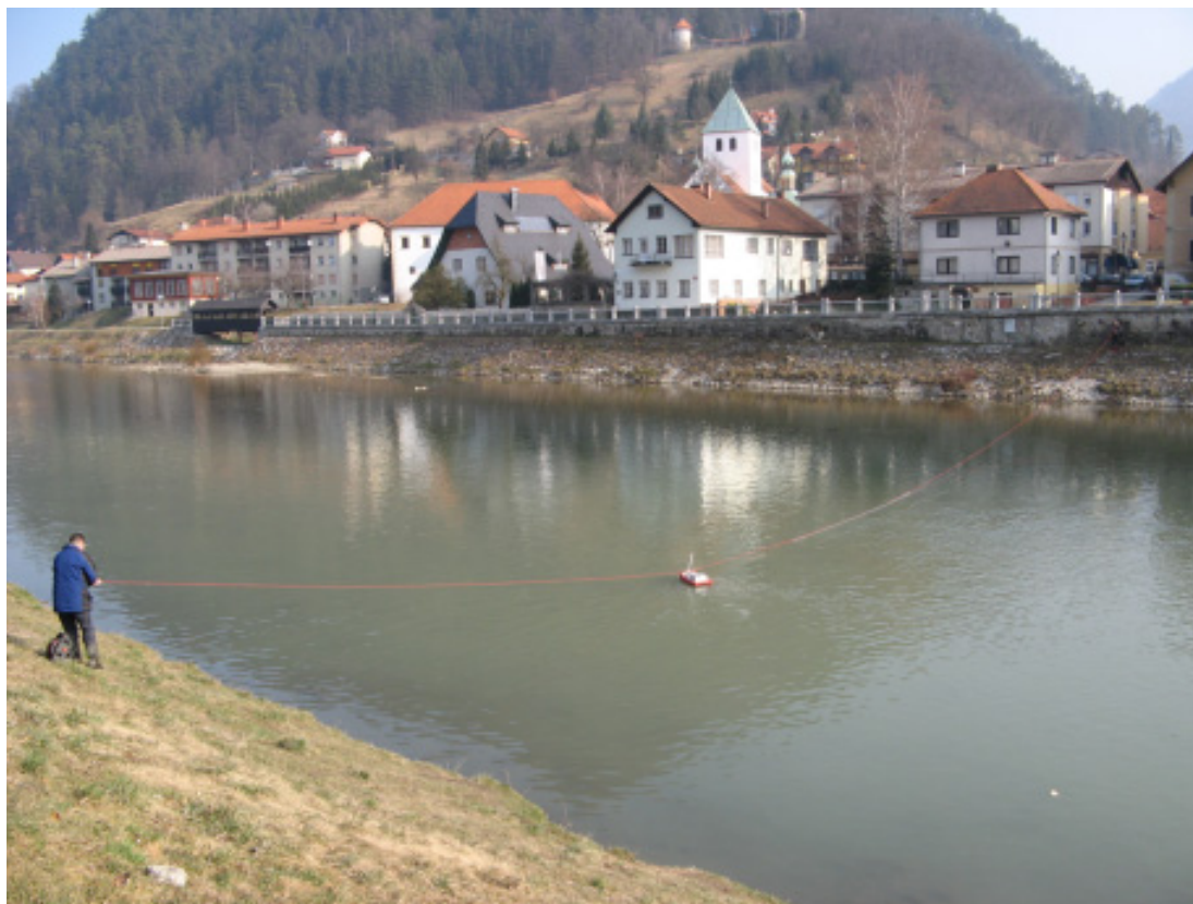
Slika 8. Izvajanje meritve pretoka na vodomerni postaji v Laškem (foto: Arhiv ARSO) Figure 8. Measuring of discharge on gauging station in Laško (photo: Archives of ARSO)
